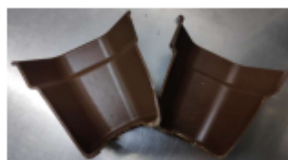
Figure 7 Demolding problems of PLARH30, at a processing temperature of 180 °C, due to a crack.
