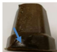
Figure 9 Big flow mark defect found in PLARH30 at a processing temperature of 200 °C.
