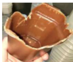
Figure 6 Short shot defect found in PLARH10 at a processing temperature of 170°C.
