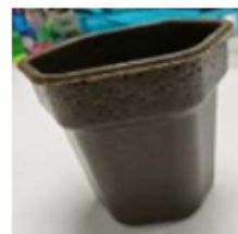
Figure 8 A good quality product of PLARH30, at a processing temperature of 190 °C, with a little sink mark.
