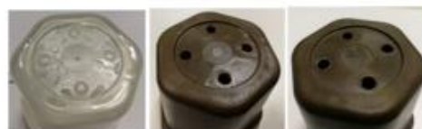
Figure 12 The sink marks (from left to right) in neat PLA, PLARH10 and PLARH30.
