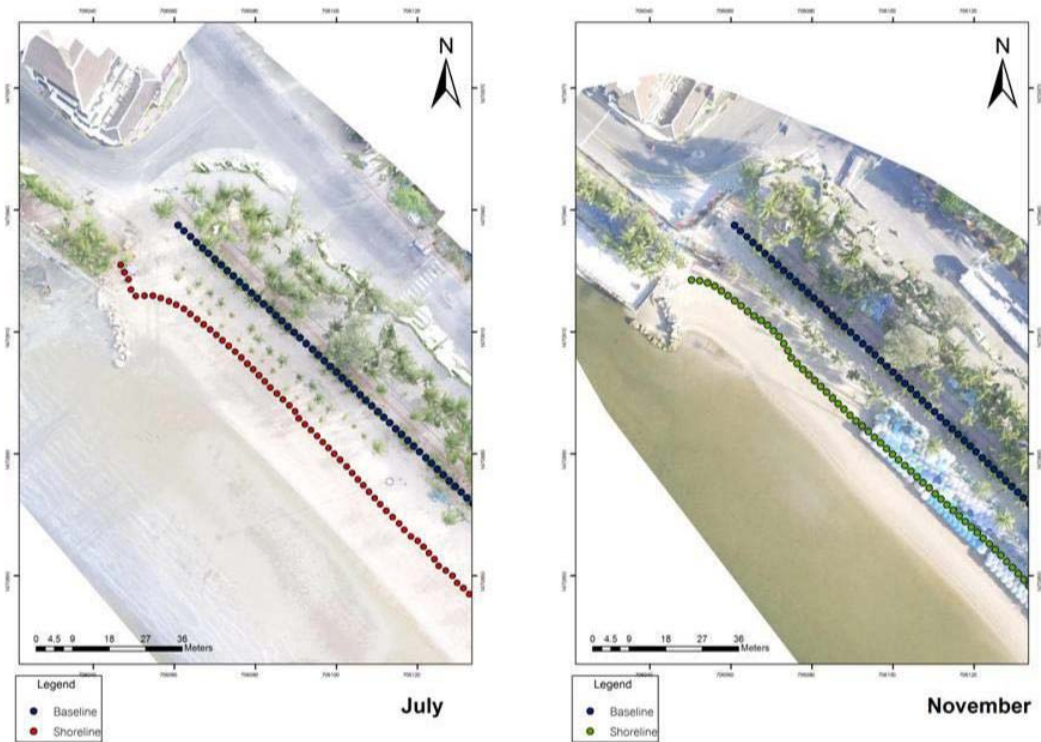
Figure 6: Shoreline mapping at Zone 1 (Laem Thaen) Blue points are baseline, red points and green points are shoreline
