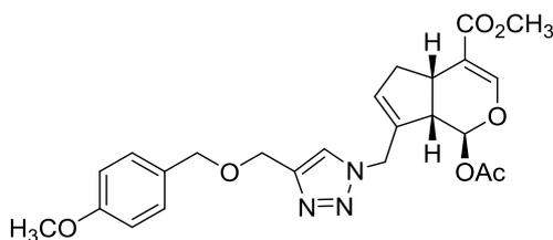
Following the general procedure, A, 4-methoxybenzyl propargyl ether (121.0 mg) was used in click reaction. The reaction was stirred at room temperature for 1 hours. The crude product was purified by silica gel column chromatography (SiO<sub>2</sub>, 40% EtOAc/*n*-hexane) to afford triazole linked genipin (**9a-6**) as a colorless oil (131.5 mg, 82%).
