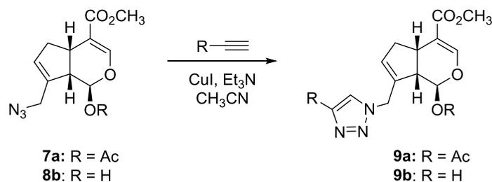
**Figure 39** The synthesis of 10-triazolylgenipin product (**9a**, **9b**)
