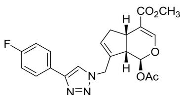
Following the general procedure, A, 4-fluorophenylacetylene (78.0  $\mu\text{L}$ ) was used in click reaction. The reaction was stirred at room temperature for 4 hours. The crude product was purified by silica gel column chromatography ( $\text{SiO}_2$ , 30% EtOAc/*n*-hexane) to afford triazole linked genipin (**9a-3**) as a white solid (109.9 mg, 78%).
