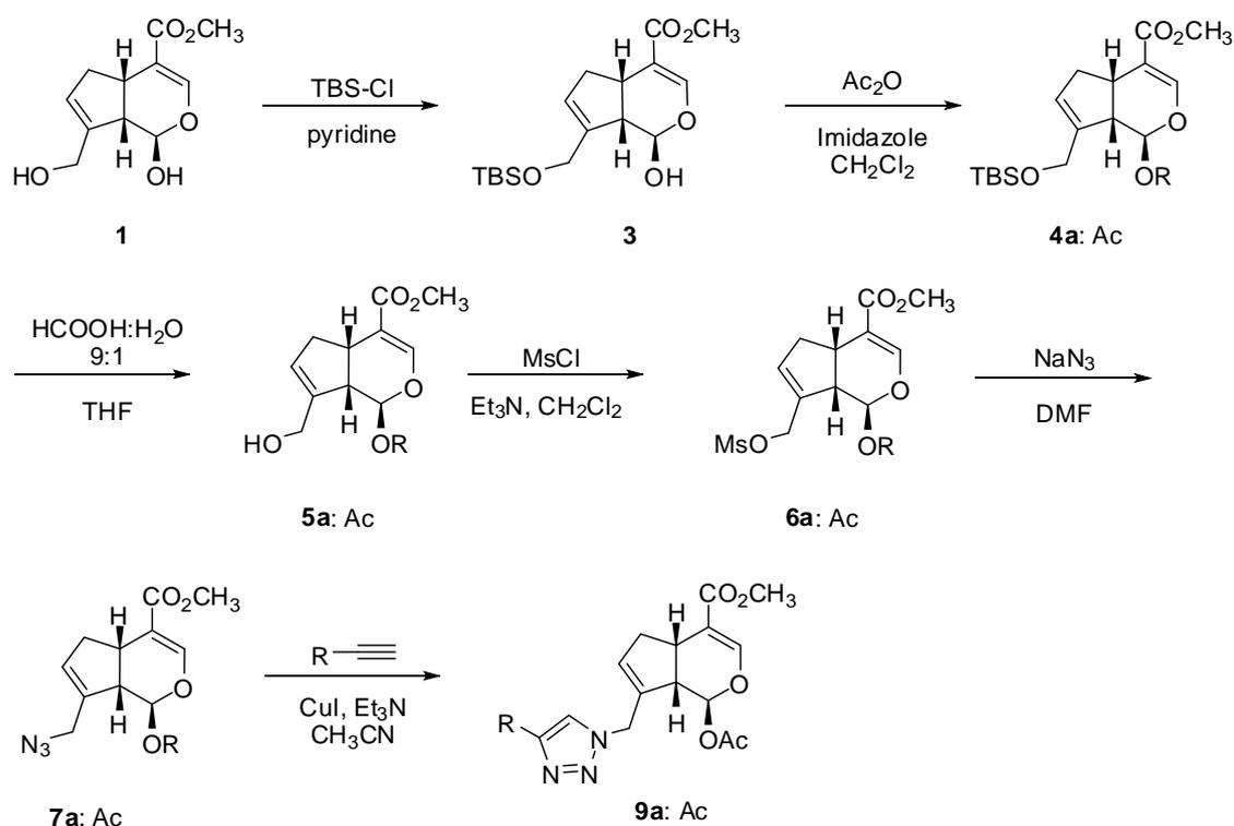
**Figure 38** Synthesis of 10-triazolylgenipin (**9a**)
