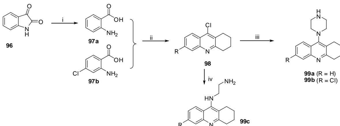
Reagents and Conditions. (i) 30%  $\text{H}_2\text{O}_2$ ,  $\text{NaOH}$ ,  $0\text{ }^\circ\text{C}$ , 3 h; (ii) cyclohexanone,  $\text{POCl}_3$ ,  $100\text{ }^\circ\text{C}$ , 3 h; (iii) piperazine,  $\text{NaI}$ ,  $\text{PhOH}$ ,  $180\text{ }^\circ\text{C}$ , 3 h; (iv) ethane-1,2-diamine,  $\text{NaI}$ ,  $\text{PhOH}$ ,  $180\text{ }^\circ\text{C}$ , 3 h.
