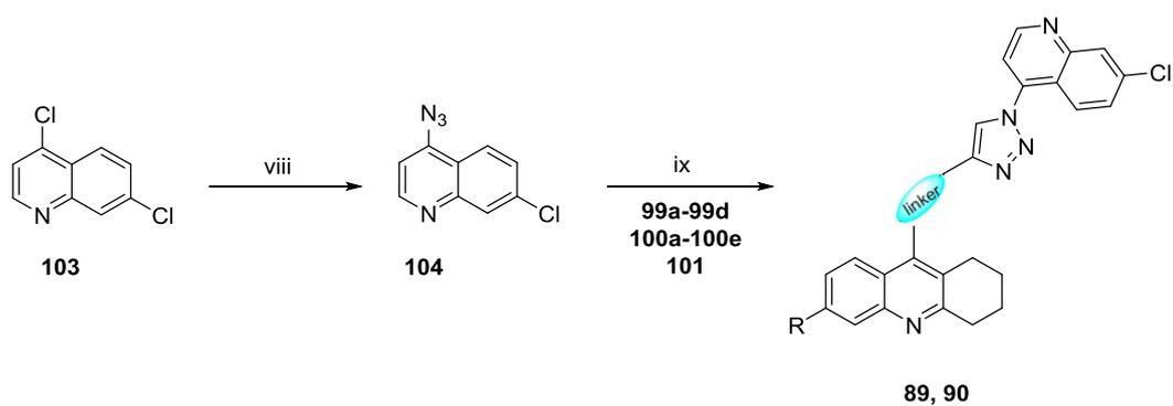
Reagents and Conditions. (viii) NaI, NaN<sub>3</sub>, DMF/H<sub>2</sub>O (v/v = 1:1), 80 °C, 8 h; (ix) Sodium ascorbate, CuSO<sub>4</sub>, Et<sub>3</sub>N, *n*-butanol/H<sub>2</sub>O (v/v = 1:1).
