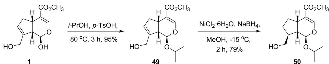
**Figure 18** The stereoselective reduction of 1-*O*-isopropoxygenipin.
