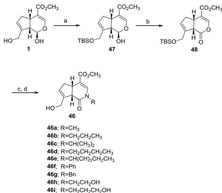
Reagents and conditions: (a) TBSCl, imidazole, DMF, rt, 1.5 h, 80-95%; (b) DMP, CH<sub>2</sub>Cl<sub>2</sub>, rt, 75-85%; (c) pyridine, RNH<sub>2</sub>, 60-130 °C; 2 h; (d) TFA, THF, 60-80 °C, 2 h, 50-70%.
